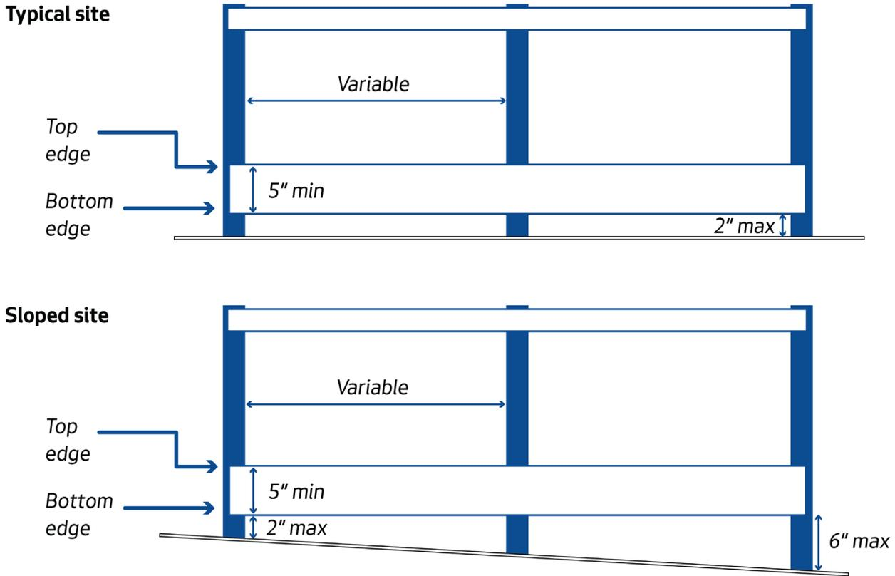
6.4.2.2 A continuous, firm barrier at 27 inches or less above the ground. If the fence or boundary element is not continuous or consists of posts connected by hanging ropes or chains, a firm detectable barrier shall run continuously along the pedestrian-side of the fence or boundary element at a height of 27 inches or less as shown in Figure 8;
